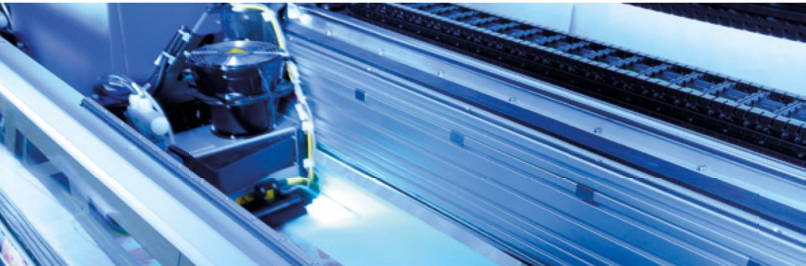
**UV curing inkjet is quickly becoming the technology of choice for the production of superwide graphics. It has enabled industrial inkjet to reach new levels of productivity and versatility as UV inkjet is instant curing and the process is clean, efficient and waste is minimised.**
